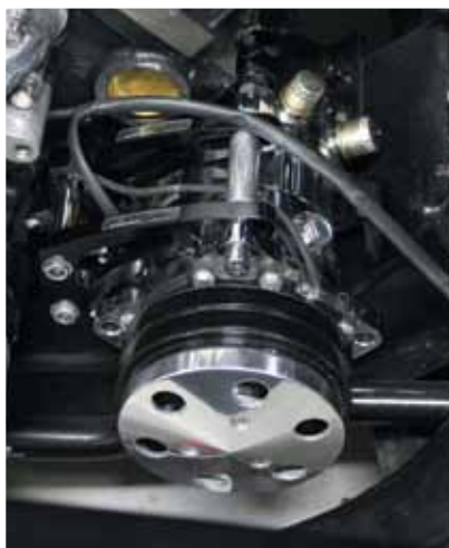
AF64-4002BLK, AF64-4012BLK & AF64-4011BLK fitted to S/B Chev in 1969 Camaro (Tall engine mounts)
