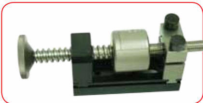
Place the stainless steel braided hose into the hose clamping mechanism and tighten the two screws to hold it in place.
