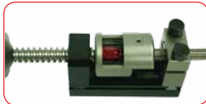
Place the socket nut into the tool holder and the hose into the hose clamp. Place the nut into the nut clamping mechanism and slide the cover closed.
